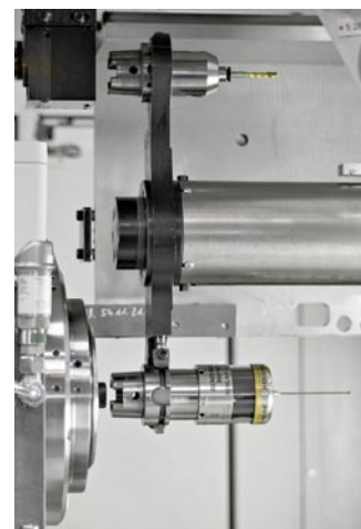
An example of a 52-fold tool changer, with the changing process being intended for the complete processing of complex components in one clamping
