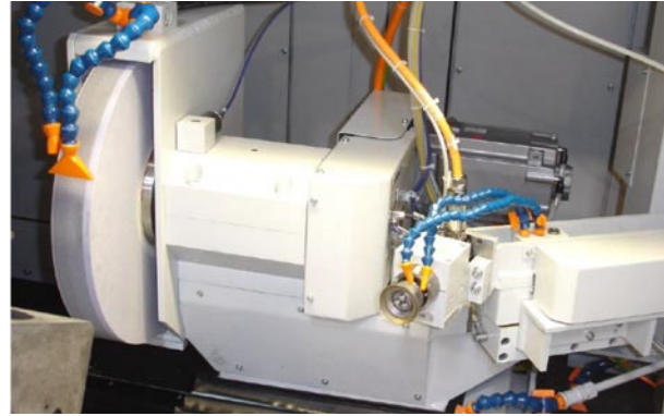
An example of an external and surface grinding unit at an angle of 90° in relation to the work-piece axis with a straight (cylindrical) external grinding wheel
