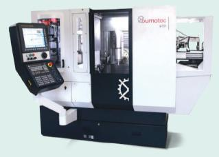
The s191 is a complete machining solution making it possible to work with bars (Ø32/50/65 mm) or blanks, rapid linear axes and a spindle reaching 30,000 rpm in under 2 seconds, a total of 7 axes, 3 spindles and 90 tools – in short, the Holy Grail.
