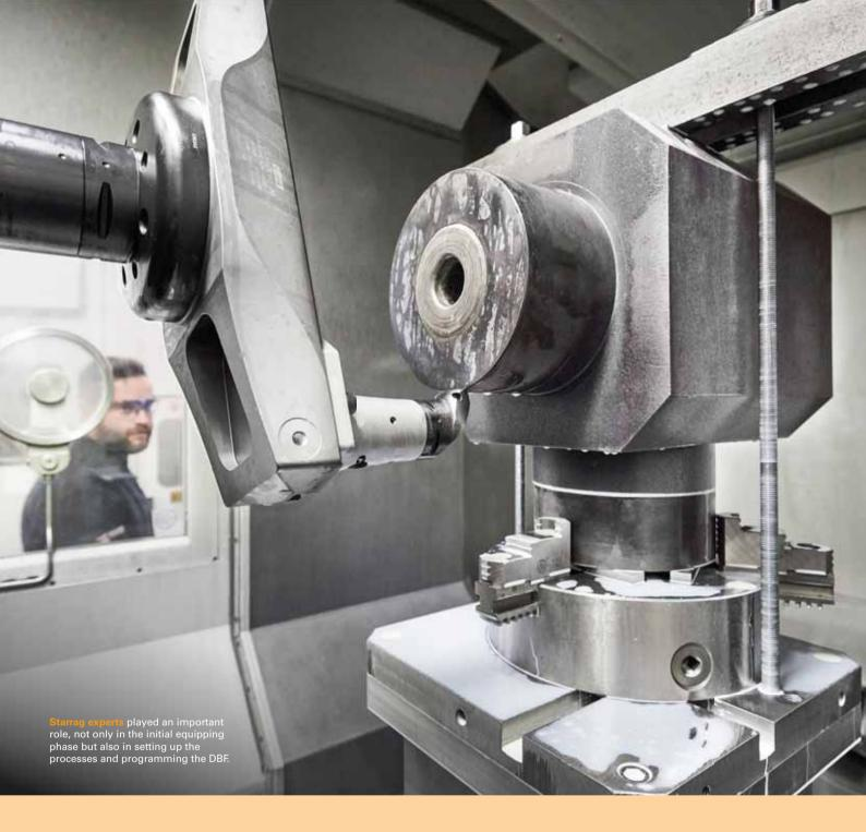
by +/- 70 mm. In addition to external, internal and face turning, the head also permits conical and contour turning courtesy of the radial facing slide's NC axis. For milling and drilling, the work spindle is arranged in its central position.
