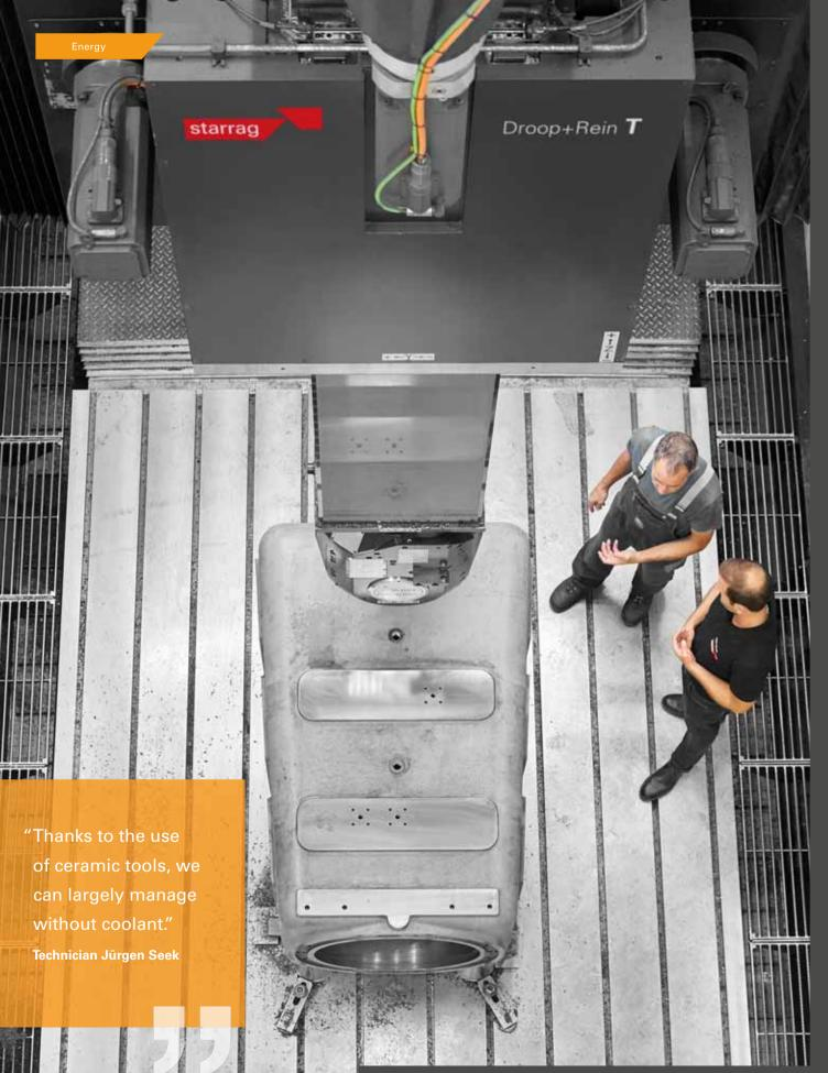
The strength of the Starrag Droop+Rein T portal machining centre lies in complete machining, which is performed with or without coolant depending on the workpiece. Minimal-volume lubrication, however, is not required owing to the high-strength materials.
