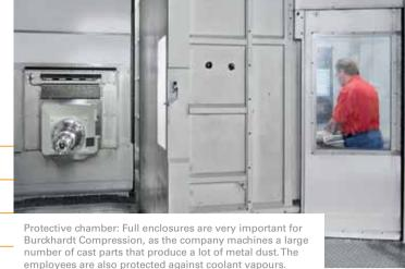
Protective chamber: Full enclosures are very important for Burckhardt Compression, as the company machines a large number of cast parts that produce a lot of metal dust. The employees are also protected against coolant vapours.
