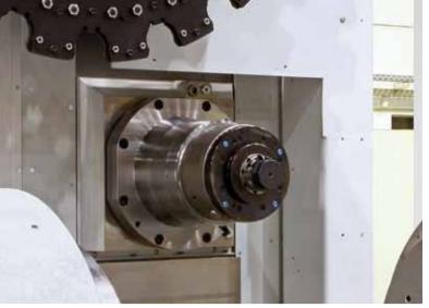
"At the heart of the machine is the spindle, available in many different versions."
