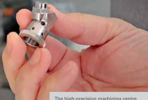
The high-precision machining centre Bumotec s191 Linear used a micro-mechanical sample piece to show off its wide range of processing capabilities.
