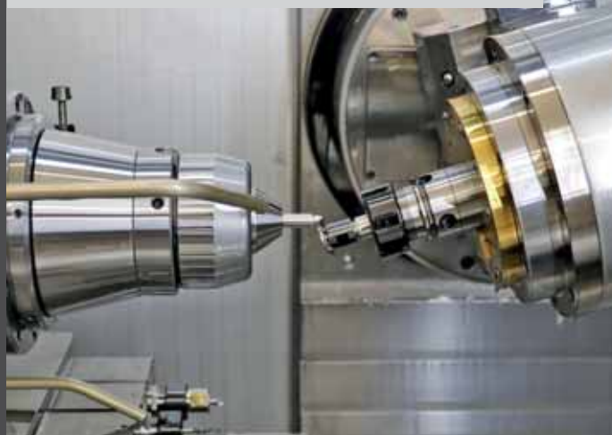
This abutment is only a few millimetres in size with very close dimensions. The s181 completely processes pieces in record breaking time. Most importantly, this offers the option of using a counter unit to process the rear side at the same time.
