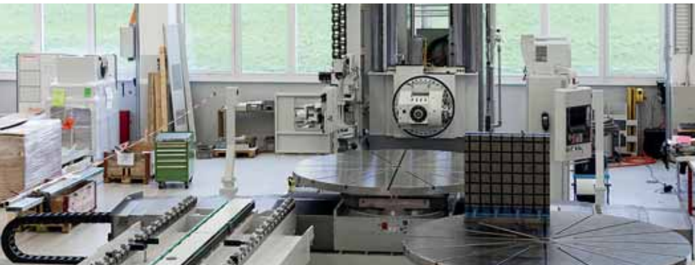
Starrag STC machining centres are now also available as MT hybrid versions. All milling and turning work on demanding structural components, multi-blades and casings can thus be done in one clamping operation.
