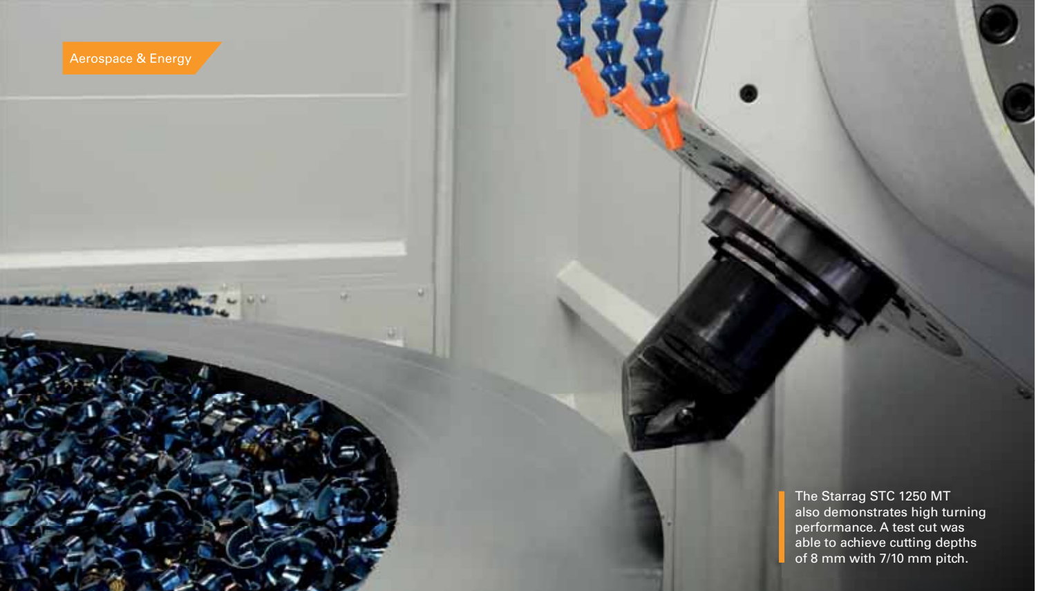
Starrag STC machining centres are now also available as MT hybrid versions. All milling and turning work on demanding structural components, multi-blades and casings can thus be done in one clamping operation.
