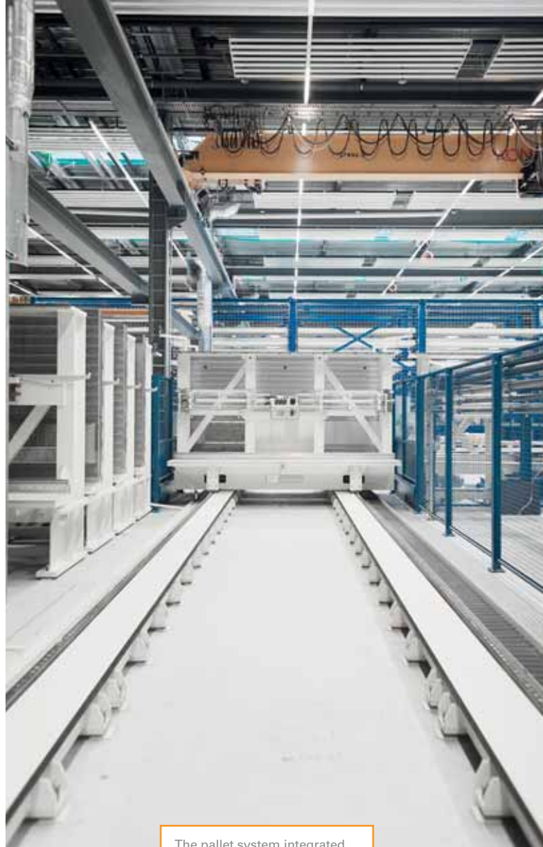
The pallet system integrated by the Starrag Group includes a total of 16 pallets measuring 2,000 mm x 4,000 mm.
